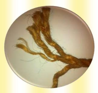
This is a photograph of some *hemp rope*. It is made from Cannabis sativa plants, grown for the strong fibres in the plants stem. Each natural material gives different properties to the rope. Hemp rope does not stretch as easily as coir rope.
