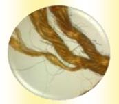
Finally the three strands get twisted into a rope.
